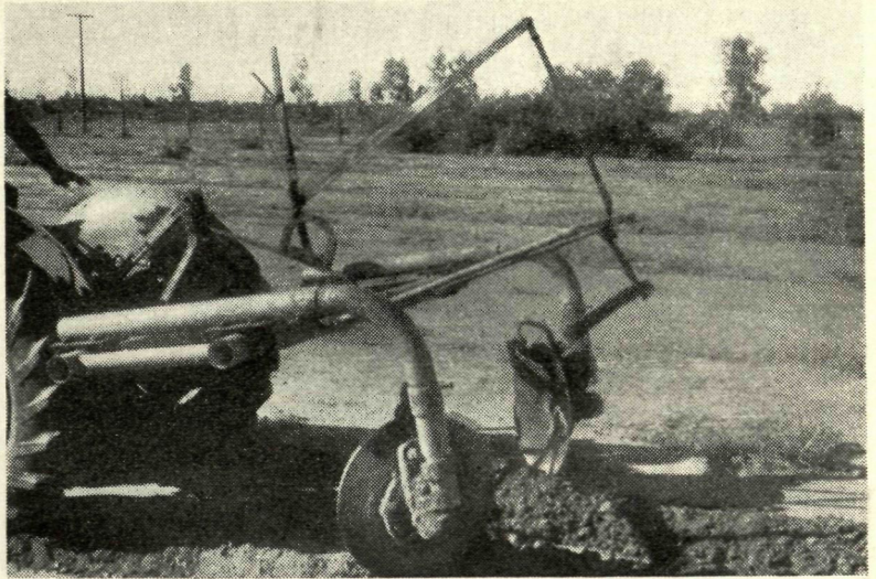
Fig. 1.—The Gascoyne Research Station "crowder"—constructed for work in cultivated irrigation soils
