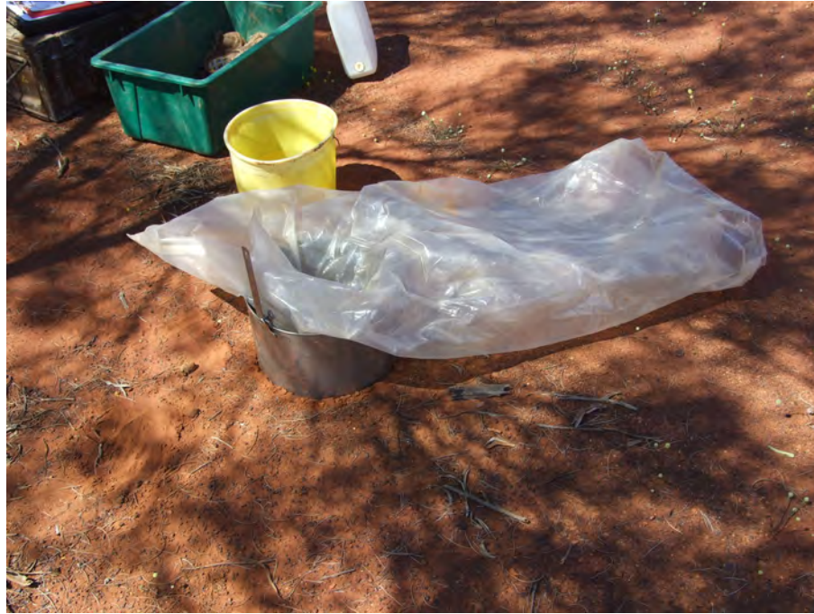
Figure 5 Infiltration ring, steel rule and plastic sheet
