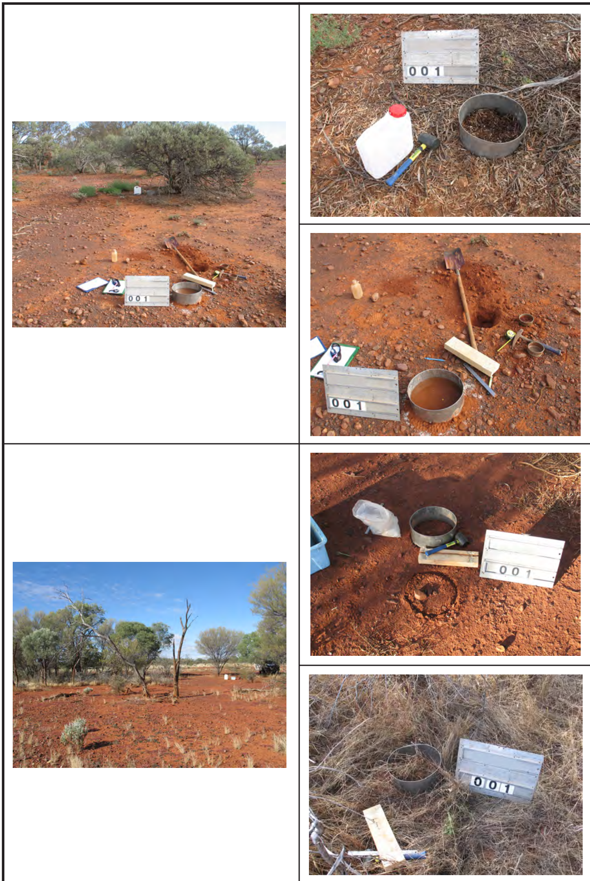
Figure 23 Examples of different resource capture zones where comparison infiltration site measurements were undertaken on interpatch and patch surfaces
