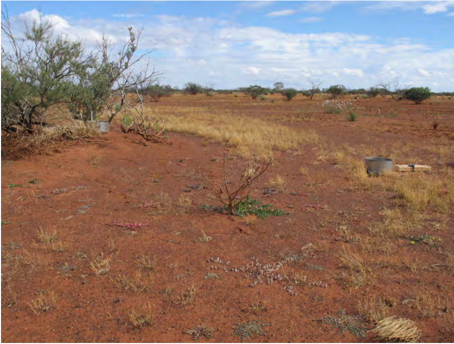
Figure 48 A soil infiltration site assessing the infiltration in a remnant interfluvial bush mound and a stripped interpatch
