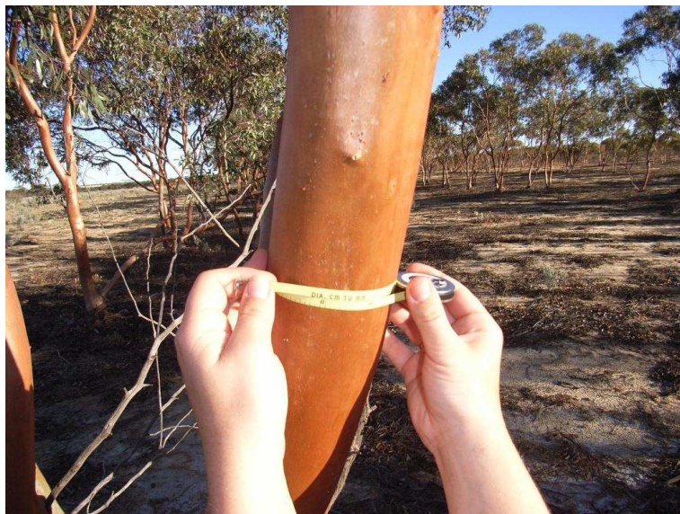
Figure 7. Stem diameter measurement with a diameter tape.
