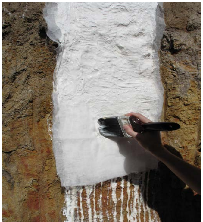
Figure 3 Use a paint brush to fix the 30 x 30 cm fabric and latex to the soil profile, ensuring no air bubbles and a good contact with the soil face.
