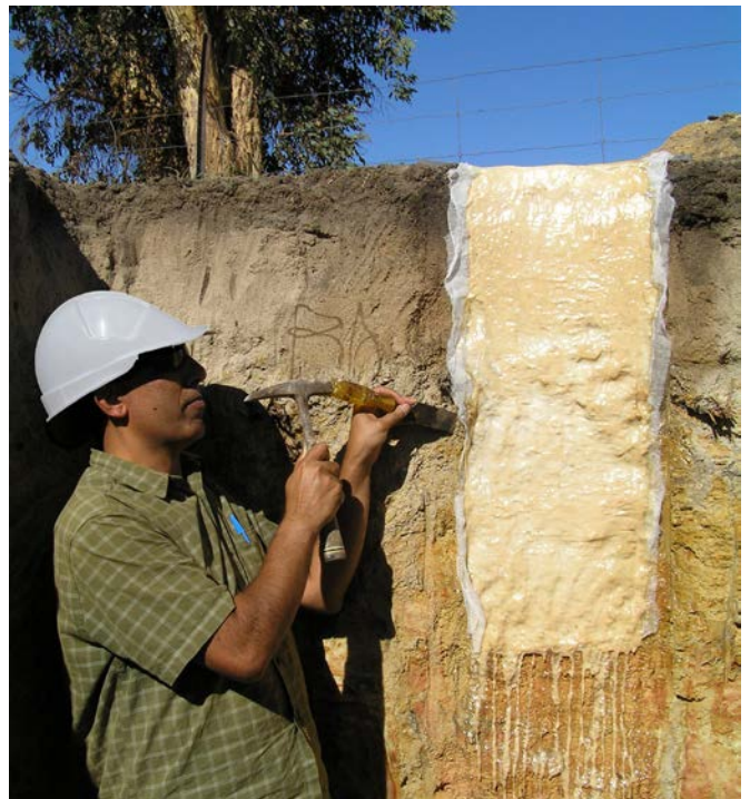
Figure 6 Removing a soil peel requires chiselling, chipping and scratching around the peel, starting from the bottom and sides
