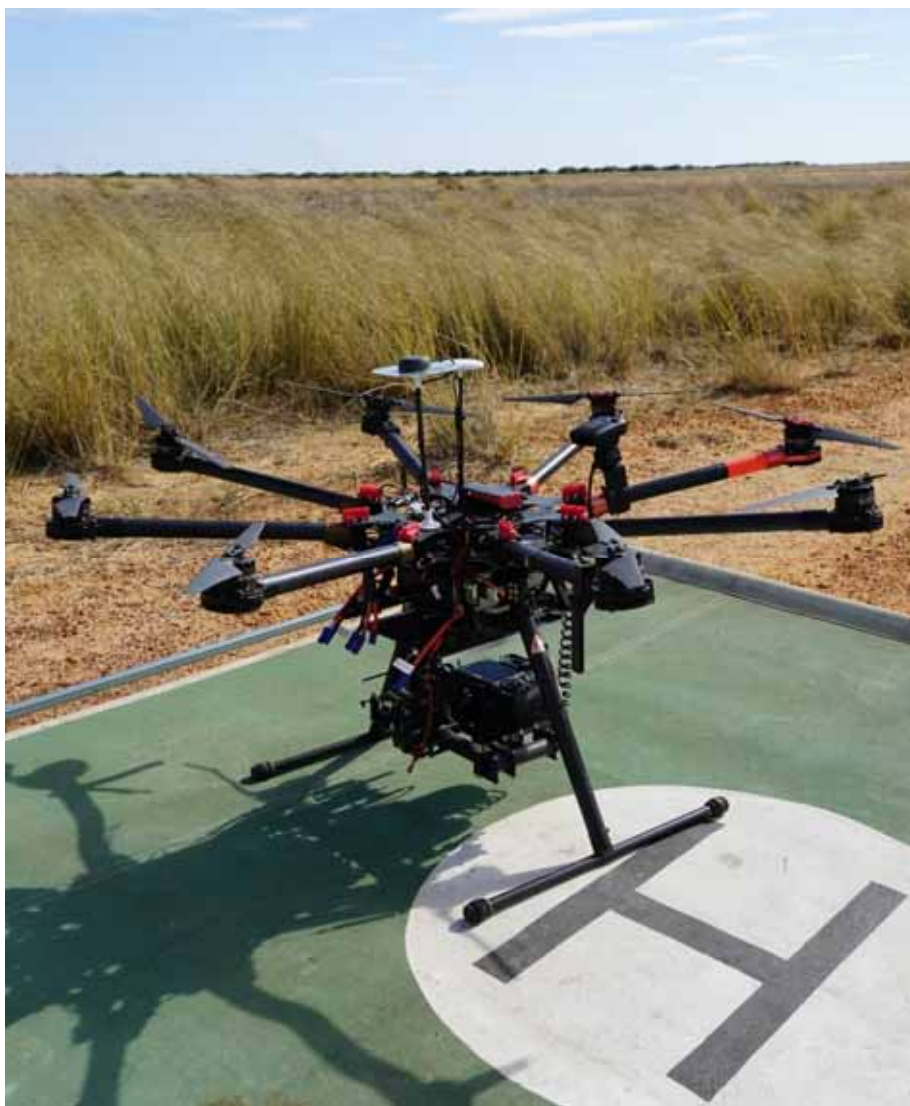
Image 8 – Multi-rotor drone used to capture aerial images
