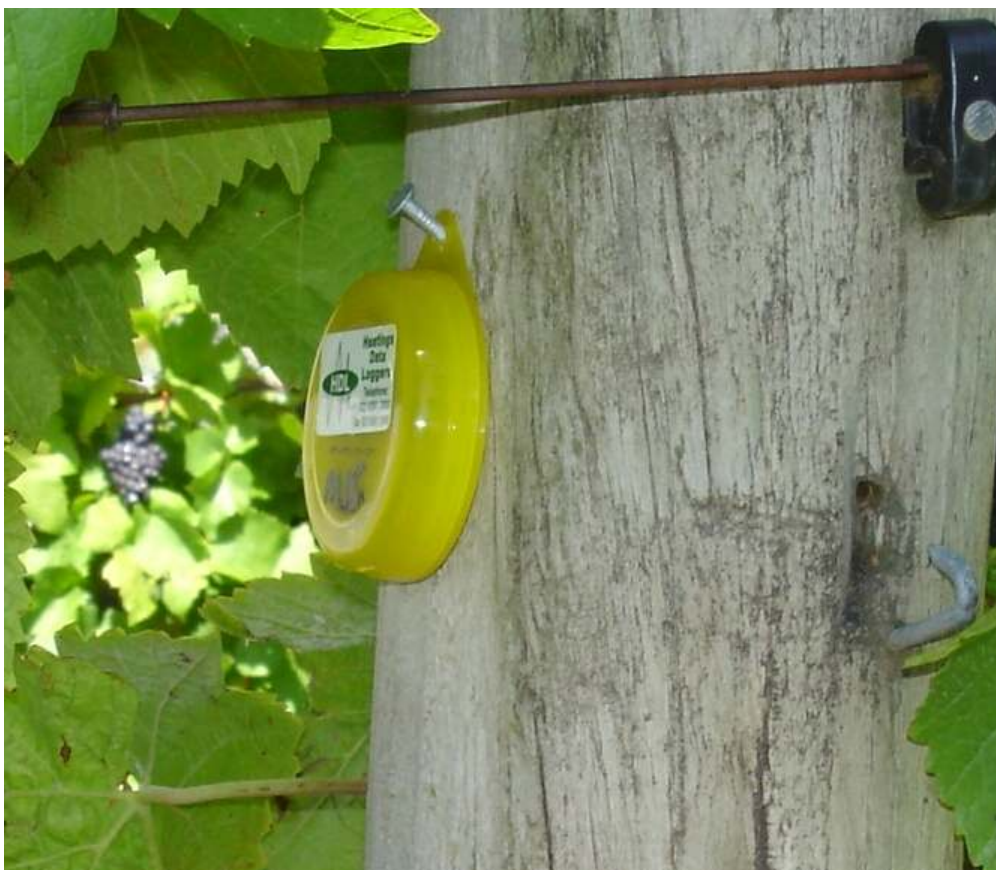
Figure 11 Tiny tag ® temperature datalogger measuring and recording bunch zone temperature in the grapevine canopy (Winter. et al. 2007)
